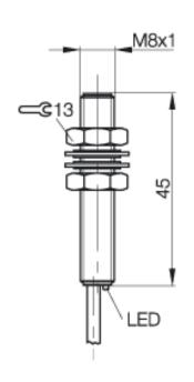
**Inductive Sensors** BES 516-343-EO-C-PU-03 M8x1 x 46.5 normally-open Sn=1,5mm shielded
